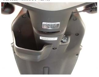
3. TURN THE MAIN SWITCH TO "ON"4. WHEN THE THROTTLE IS TOTALLY CLOSED, HOLD THE BRAKE LEVER&PUSH THE START BUTTON OR USE THE KICKSTARTER TO START THE ENGINE.
