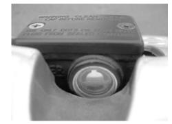
WHEN CHECKING THE OIL LEVEL, PLEASE TURN THE HANDLE BAR ASSURING THAT THE BRAKE OIL IS IN HORIZONTAL POSITION.
