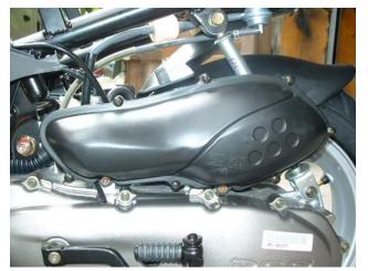
PREVENT THE ASH ENTERING THE ENGINE AND WEAR OUT THE ENGINE. PLASE ASK THE DEALERS TO CHECK & CLEAN THE FILTER FOR THE TIME BEING.
