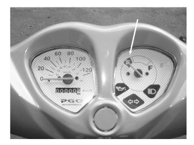
NOTE: WHEN SWITCH OFF, THE INDICATOR WILL POINT AT THE "E" POSITION.
