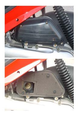
NOTE: PLEASE DO NOT START THE ENGINE BEFORE THE AIR-CLEANER IS ASSEMBLED, OTHERWISE THE ENGINE WILL BE BADLY WORN OUT.
