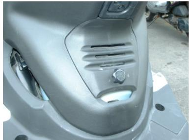
6.Screwing out the screws of left side cover
