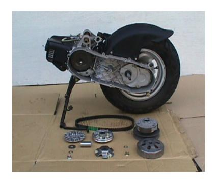
7. Loosen 2 hexagon screws, and take off the driving gear starter fixing plate set.
