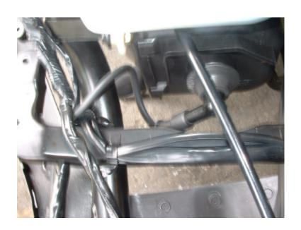
5.Remove engine hanger shelf's nut, rear damper blot and rear brake cable.
