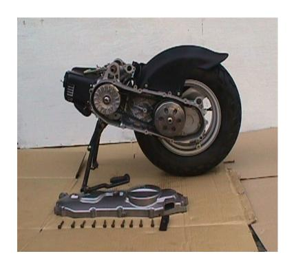
3.Remove the fixing nut of clutch.
