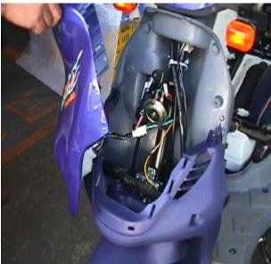
10.screwing out the screws of front inner cover.
