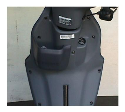
11.screwing out the screws of front mudguard.
