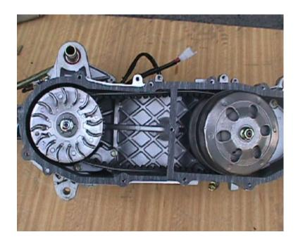
4. Take off the ramp plate, belt & rear clutch, and the driving plate.
