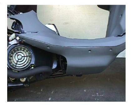
Locking torque: M6:0.7-1.1kg-m M5:0.35-0.5kg-m
